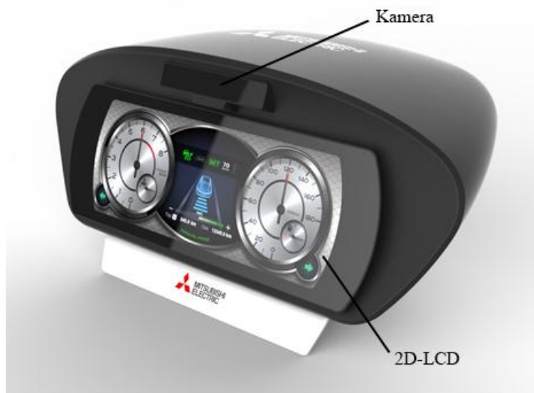
Real Texture implementert i et bilinstrumentpanel
